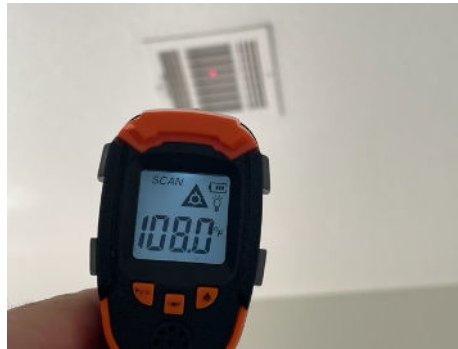
108 Degrees- Recorded hot air supply temperature
