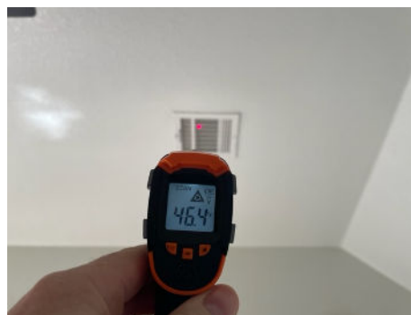
46 Degrees- Recorded cold air supply temperature
